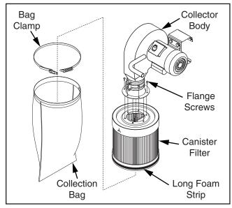
**Figure 7.** T10877 final assembly on dust collector.
